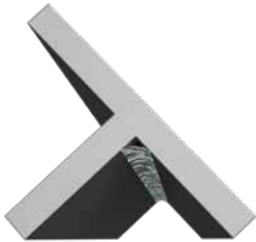
Tee Joint (Overhead 4F)
