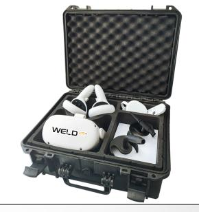
To get started open up the WeldVR hardcase and take out the Oculus Quest 2 Headaset, Controllers, Controller Mount and Google Chromecast.
