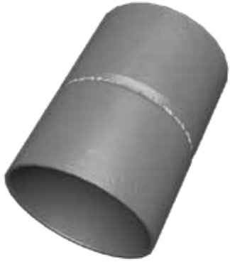
Pipe to Pipe Joints (6G)
