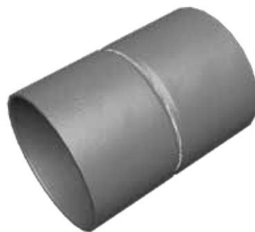
Pipe to Pipe Joints (1G)
