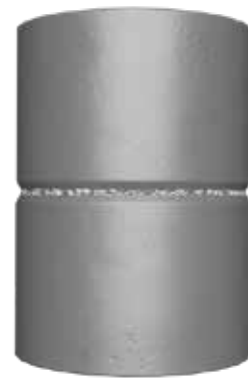
Pipe to Pipe Joints (2G)
